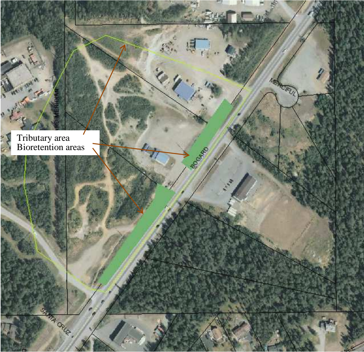
Figure 11: Bogard Road between Seldon Road and Seward Meridian Parkway Bioretention – Conceptual Layout
