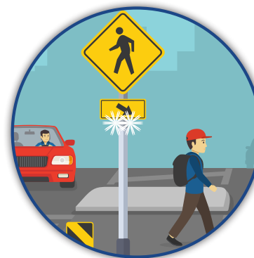
Rectangular Rapid Flashing Beacons (RRFBs)
