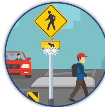
Rectangular Rapid Flashing Beacons (RRFBs)
