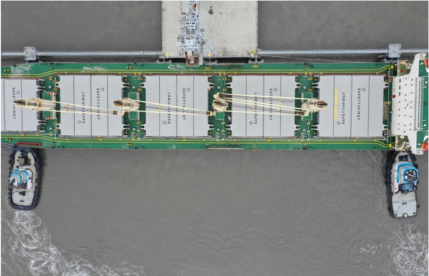
Above photo: Aerial view of tugs holding vessel in place as lines are secured.
