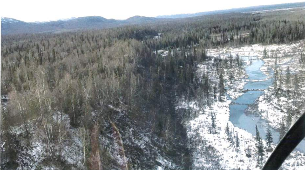
Figure 8: Skwentna River floodplain on the right and the adjacent bluff on the left. The proposed alignment at this location is through the floodplain at the toe of the bluff.
