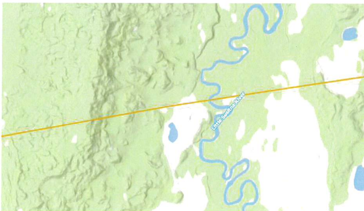
Figure 14: Hillshade map of the EWR Rail crossing of the Little Susitna River. Note the bluff on the west side of the river.
