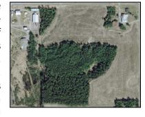
bands. Only three bands can be viewed at one time in most software applications. A user typically chooses to display an image as either natural color (red, green, and blue bands)—as shown in the example to the right--or color infrared (infrared, red, and green bands)—as shown in the example to the left.
