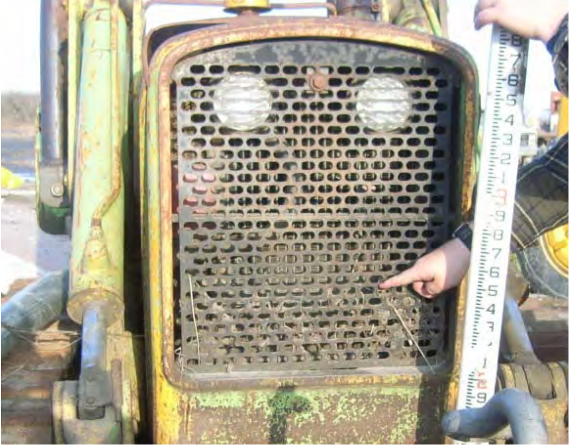
Figure 11: grass line on bulldozer grille, Good, Emmonak, 2009. Equipment may contain usable marks if it doesn't move from the time of the event to the time it is surveyed.
