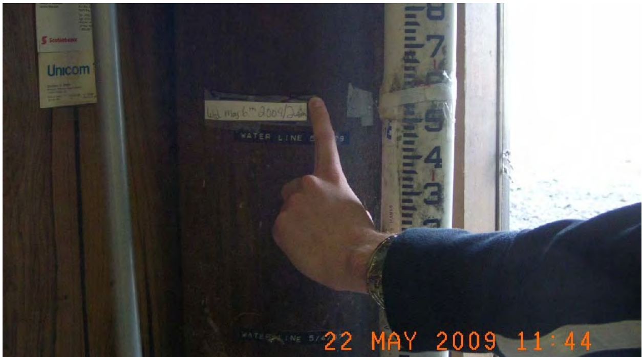
Figure 2: Durable high water mark in circle placed by building owner. A record of water levels on this post had been recorded for 20 years and all were measured during the survey.
