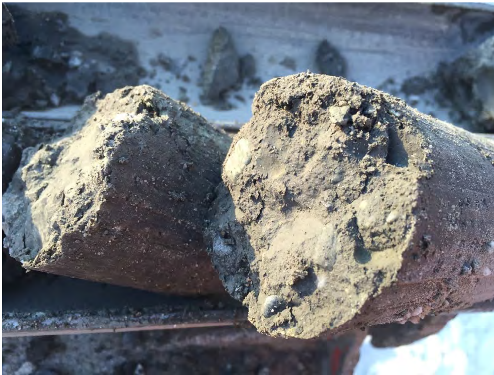
Photograph #2: Very dense silty gravel from 22-24 feet below ground surface at Church Road boring #1.
